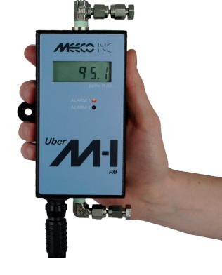
Service with a Big Smile : The Uber M-I comes with a full two-year Certificate of Calibration. The cell can easily be replaced in the field, with no need to disconnect the unit from the sample stream! Also, spare cells now have a two-year storage life if held in their unopened shipment bags.
