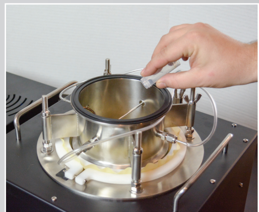
Load Step: Test dust can be easily loaded into system.
